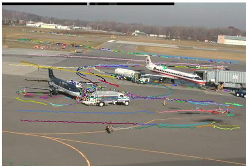
Figure 9. Tracklets produced by mean-shift tracking with automatic initialization on sequence T09.
