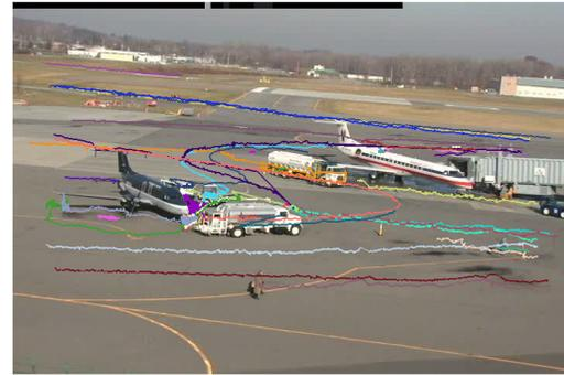
Figure 10. Results of independent track linking, *i.e.* no use of the event model, on sequence T09. The event recognition scores are poor because the actor tracks are still partially fragmented. For example, the driver/refueler is fragmented into the purple, green and violet tracks near the front and right wing of the plane.
